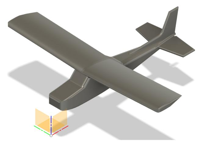
The wing span is just short of one meter and about 750mm nose to tip, so this needs to be chopped up in parts that will fit on my 3D print bed of  $230 \times 230 \times 250$ .
