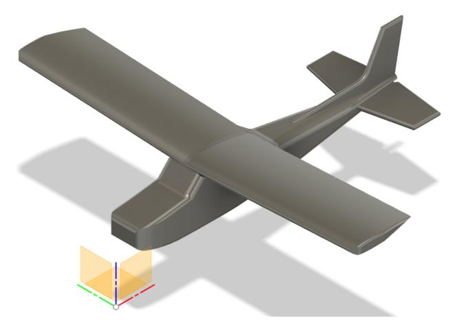
The wing span is just short of one metre and about 750mm nose to tip, so this needs to be copped up in parts that will fit on my 3D print bed of 230 x 230 x 250.
